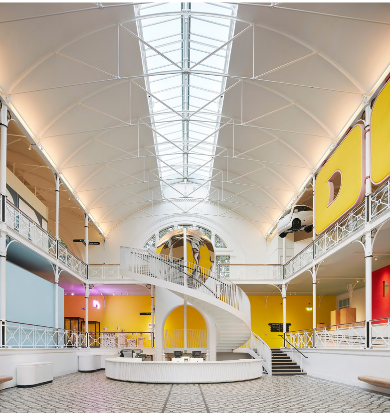
Soft warm uplighting to the barrel-vaulted roof celebrates the architecture and softens contrast, while spotlighting provides functional light and highlights key architectural features. Photos: © Hufton & Crow
